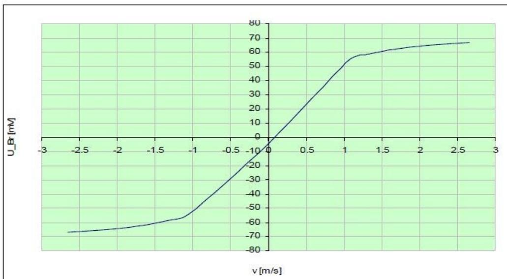
Typical signal – curve between 0 ... 2.5 m/s
